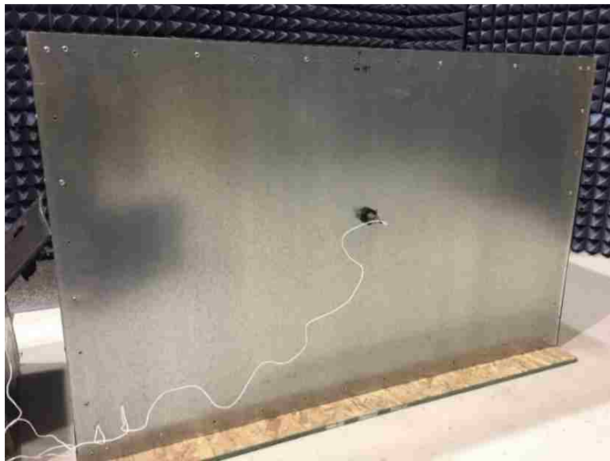
Fig. 6.6. Experimental setup to measure damped free vibration at the center of the long sidewall using an accelerometer.
